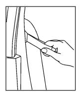
Pull the loop, located on the outboard side of the seatback, forward until you hear a click.
